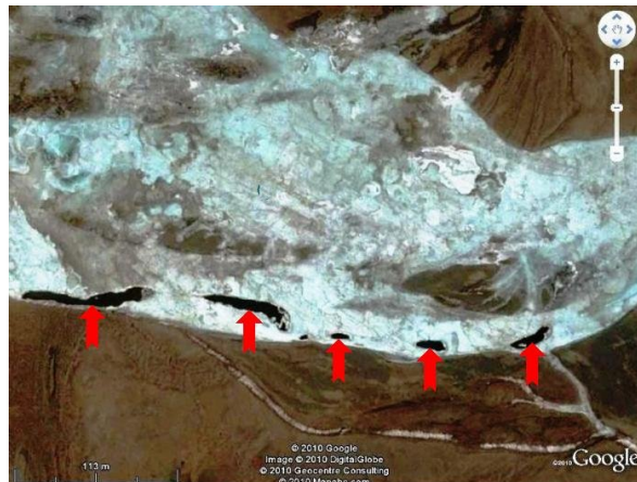
Figure 19. phreatic tube in disintegrating ice shield Unroofed phreatic ice tube containing water (red arrows). Tset floodplain, Mongolia (image: Google Earth - 9 th March 2004)
