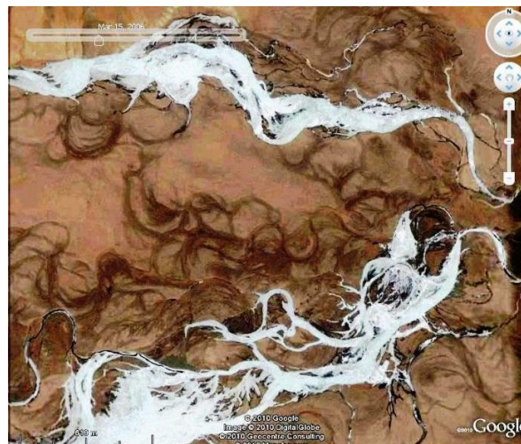
Figure 22. naleds in high-definition satellite image The scene is of naleds on river floodplains at Tset in Mongolia, showing the ease of detecting naleds in high-definition satellite images that now rival air photos but demand the skills of aerial photograph interpreters. (image: Google Earth - 15 th March 2006)
